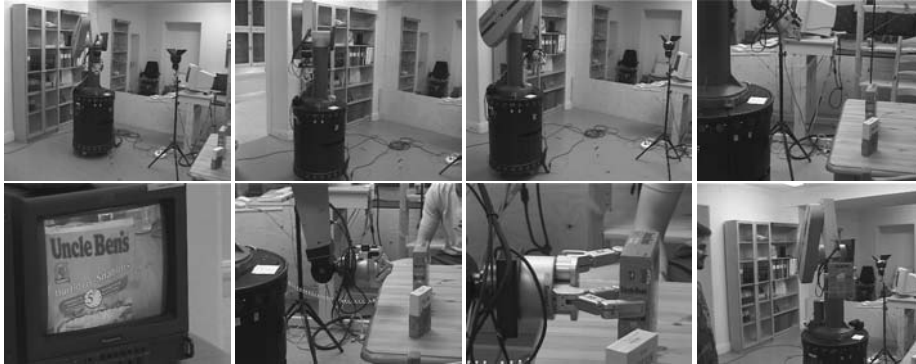
Figure 12: An experiment where the robot moves up to the table, recognizes the rice box, approaches it, picks it up and hands it over to the user.
