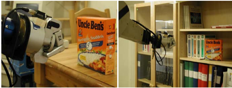
Figure 2: The left image shows the gripper in a reference position while the right image shows the camera in another position and situation. Servoing is then used to move the camera to the reference position relative to the object.
