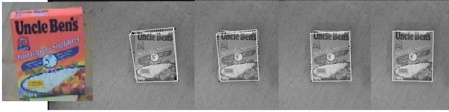
Figure 6: Training image used to estimate the initial pose (far left) followed by the intermediate images of the fitting step.
