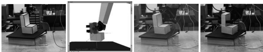
Figure 8: Grasping of the L-shaped object: The pose of the object is estimated in the camera coordinate frame (the estimated pose is overlaid in black). The pose is transformed to the manipulator coordinate system using the off-line estimated camera/robot transformation. The estimated pose is propagated to GraspIt (first row, right) where a stable grasp is planned (the measures of the quality of the grasp are shown in the lower left corner of the image: e=0.317 and v=1.194 ). The planned grasp is used to position the manipulator and the hand.
